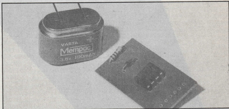
Above: Clock battery backup, Rainbow Digital
